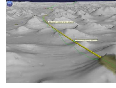
Solving engineering challenges in global response analysis of subsea pipelines and cables by including 3D non-linear time domain VIV analysis of free spans.
